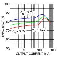
The Figure above shows an efficiency curve. From 1µA to 100mA, efficiency losses are dominated by quiescent current losses, gate drive and transition losses. By using the HyperLight Load<sup>™</sup> mode, the MIC33050 is able to maintain high efficiency at low output currents.
